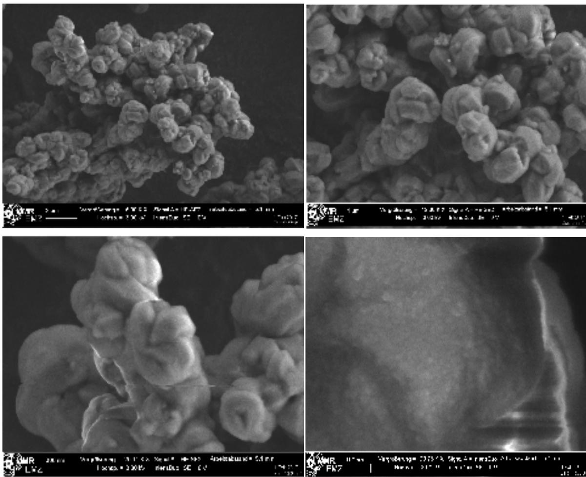
**Figure 30:** SEM images showing the morphology of SBA-15.
