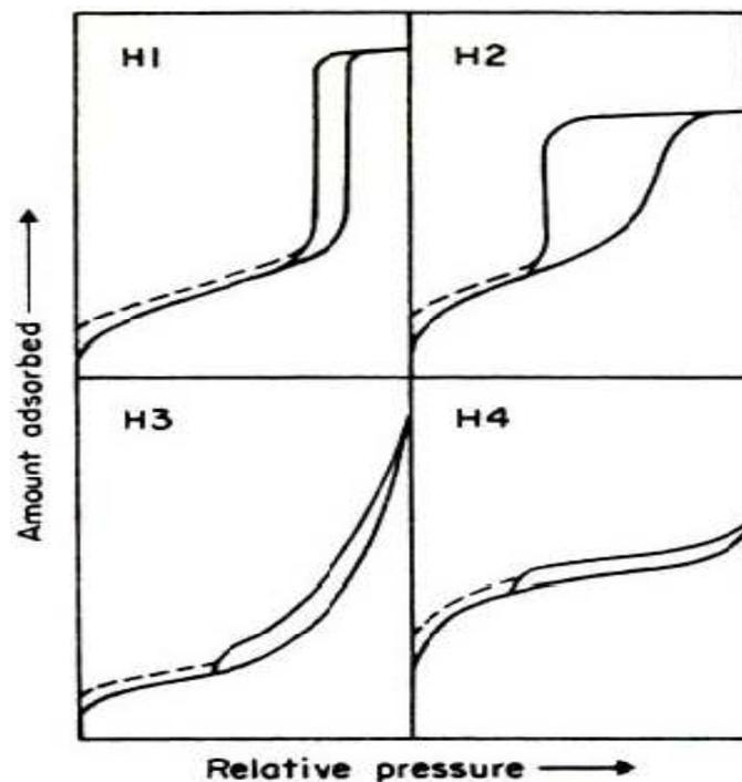
**Figure 4:** The four main types of hysteresis loops according to IUPAC classification. <sup>[60]</sup>
