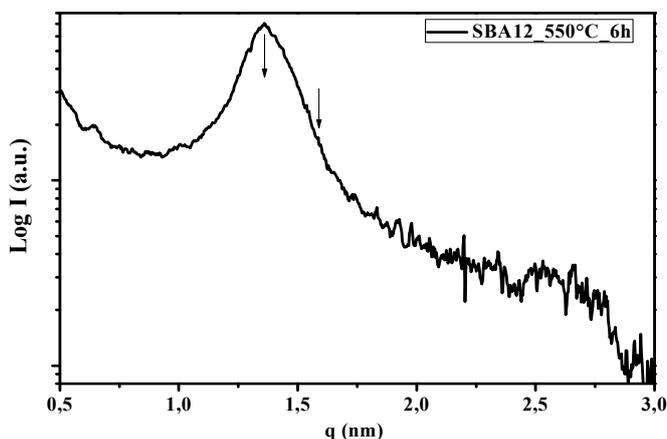
**Figure 35:** SAXS patterns of the calcined SBA-12.
