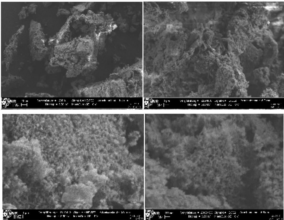
**Figure 23:** SEM images showing the morphology of MCM-48-L.
