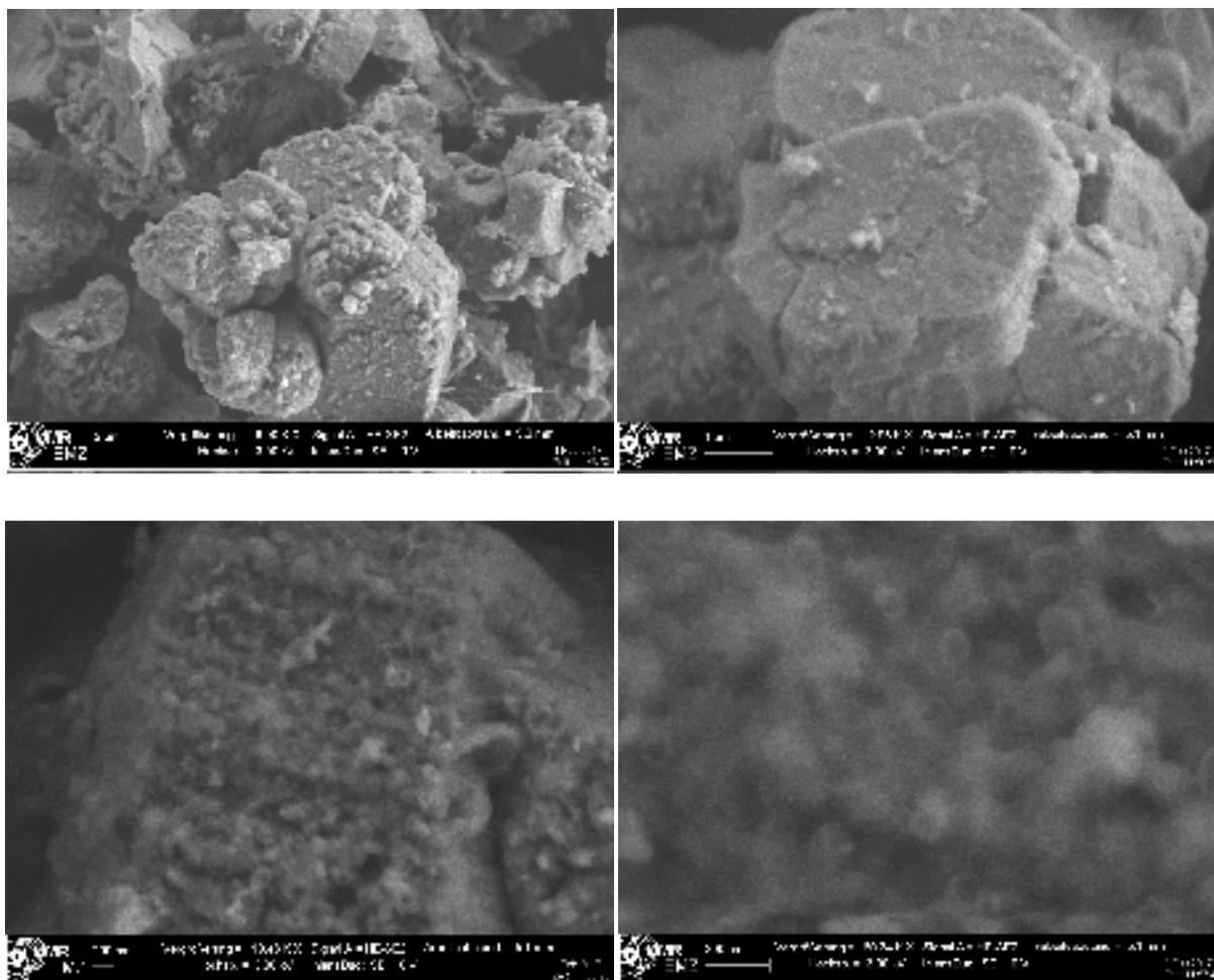
**Figure41:** SEM images showing the morphology of FDU-12-S.
