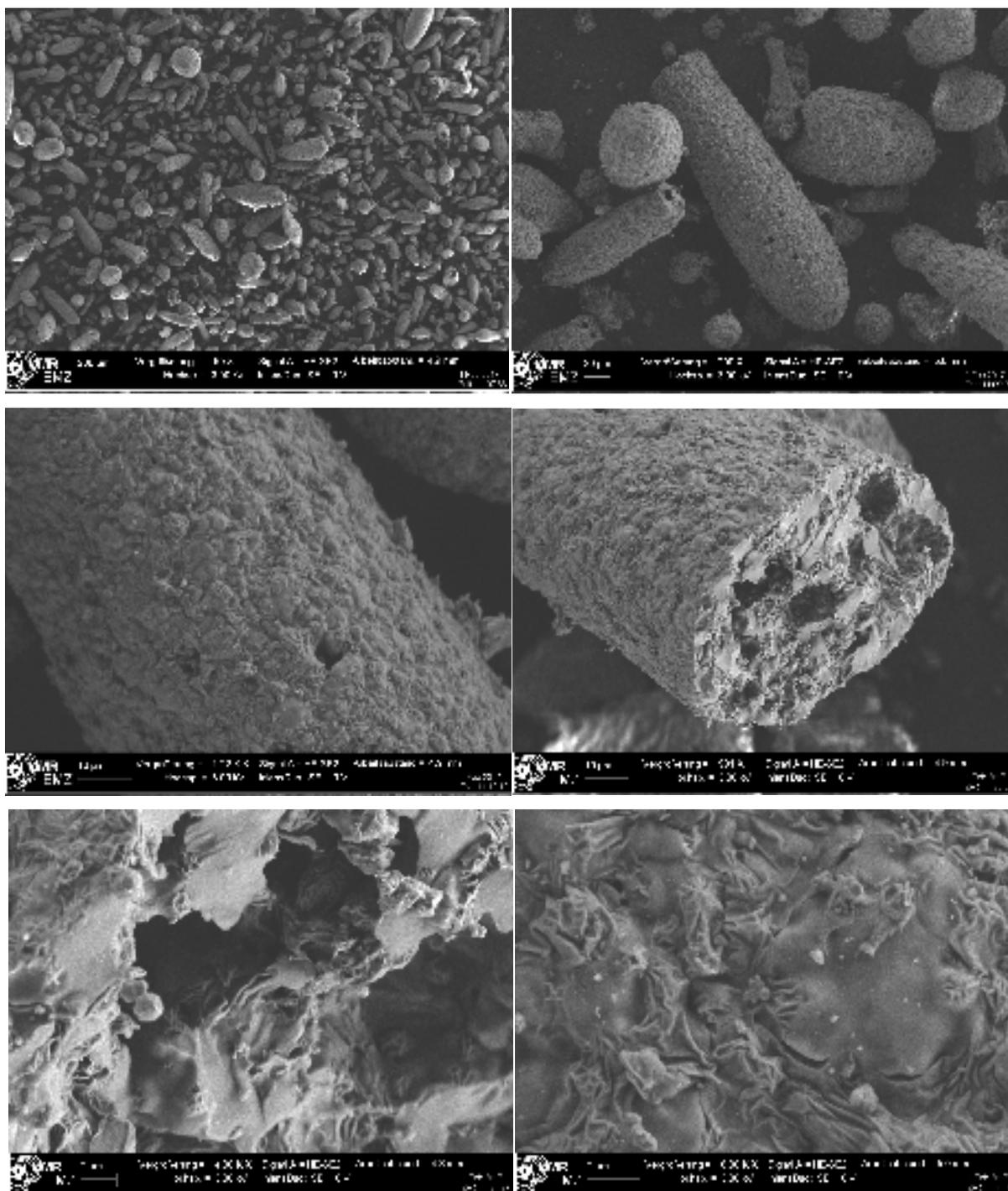
**Figure 27:** SEM images showing the morphology of KIT-6.
