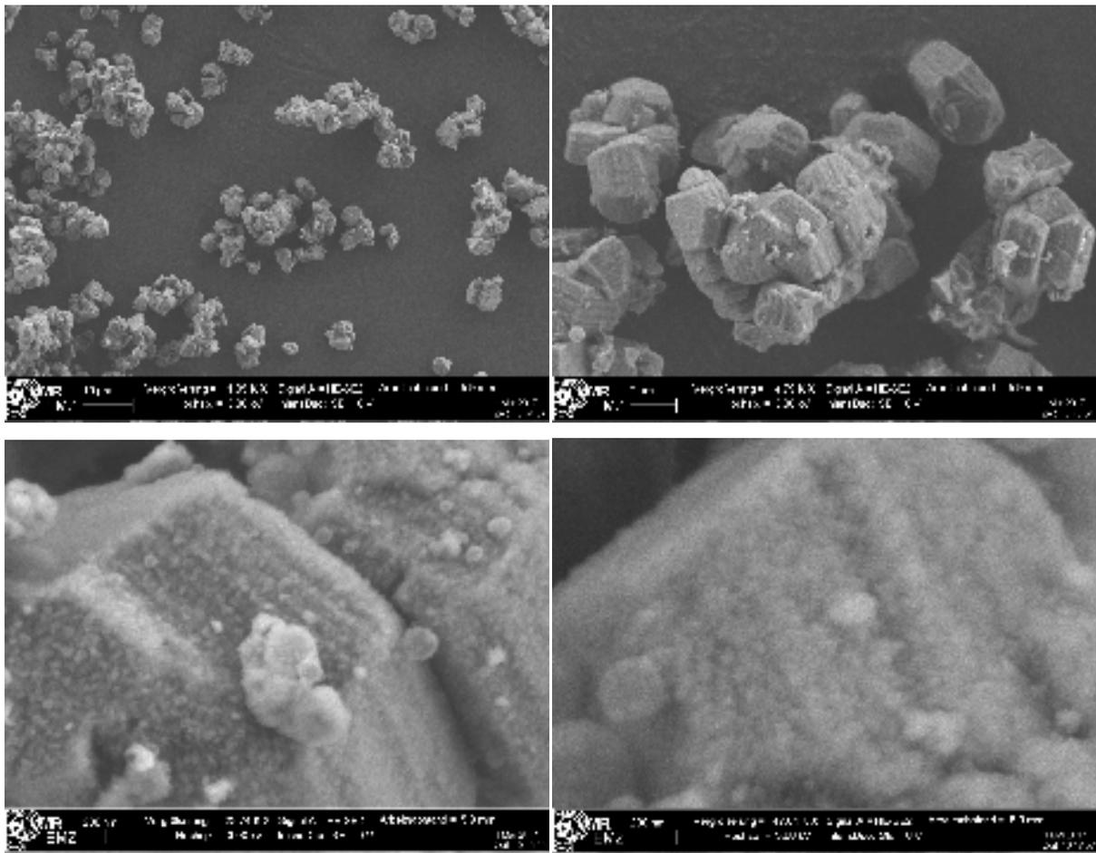
Figure 42: SEM images showing the morphology of FDU-12-L.
